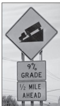
Fig. 4.7. The road grade is typically given as a percentage.
