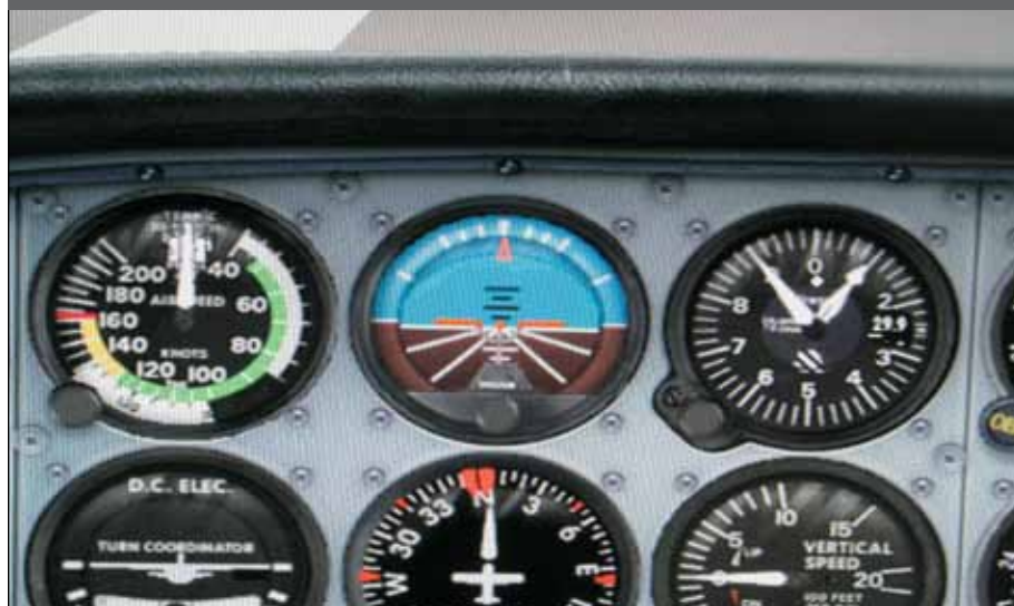
Fig. 1 It took some effort to familiarize students with how to interpret the information on the instrument panel of an airplane, specifically, from left, the air speed indicator, the attitude indicator, and the altimeter.
